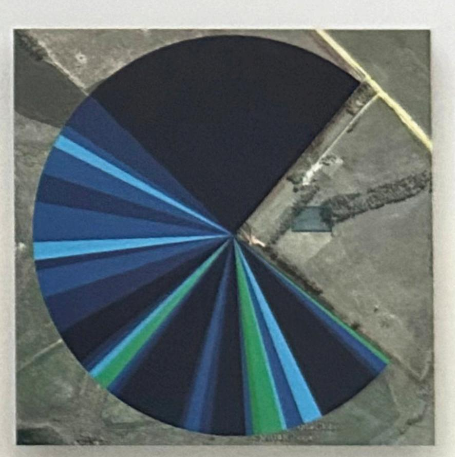
A Speed VRI Rx was easily created from the aerial image. Sectors were incrementally inserted to one-tenth of a degree to divide the field into manageable areas that can be independently controlled. The areas unaffected were colored for 100 percent application.
